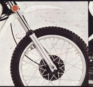
**Long travel, heavy-duty front forks** soak up sharp jolts without bottoming. Heavy-duty wheels front and rear equip the XT500 for comfort, control and durability over the roughest terrain.
