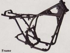
In order to give the bike better dynamic stability, the high-tensile-strength, doublecradle frame carries the engine low and forward. This tubular-steel frame is also designed to be able to withstand twisting, turning and impact stresses that are incurred on the roughest of roads so that the bike will be able to offer dependability regardless of the road conditions.
